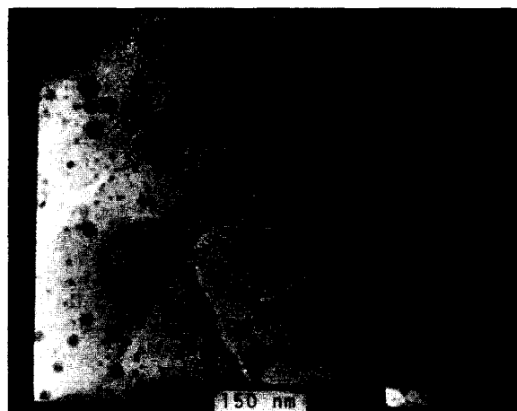
Fig. 4. TEM photograph of Ag fine particles in Ag particle-impregnated CA membrane.
